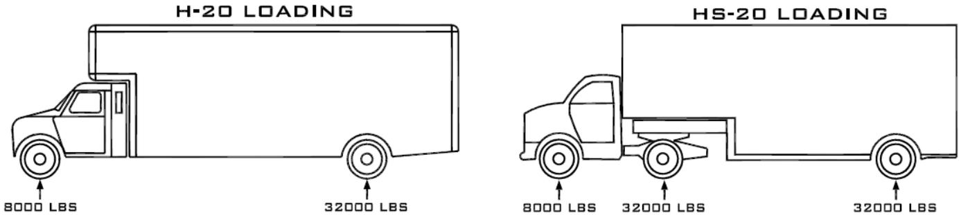
**Step #1) Determine the maximum wheel load:**
