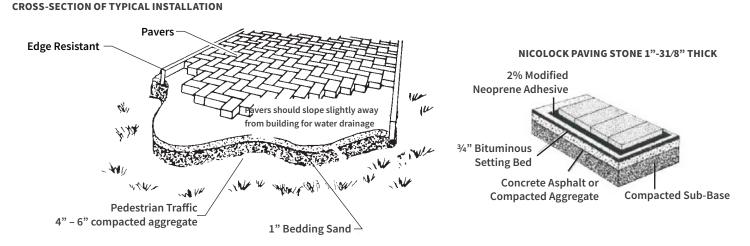
**NOTE:** All measurements are nominal. Variance in square footage or linear footage coverage can be up to 5% depending on joint width. The possible occurrence of efflorescence does not affect the structural integrity of the product. Efflorescence is a normal occurrence in concrete products and will dissipate with normal weathering. The use of concrete as a base or setting bed may increase the possibility of efflorescence.
